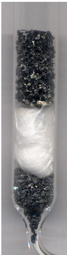
Fig. 2. Photograph of a prepared monolith into the U-shape glass reactor.
